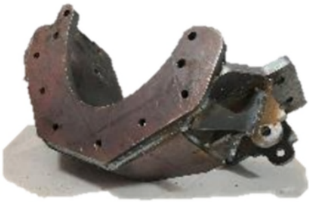
Example for type of cradle allowed and pulley protector.
