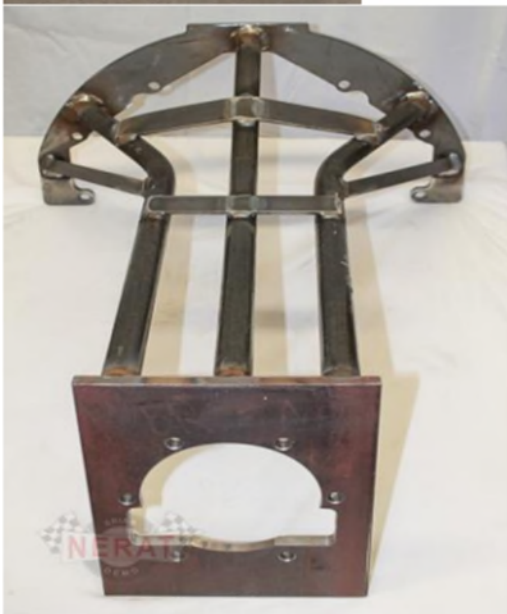
Example of trans braces allowed.
